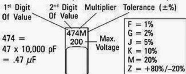
On some capacitors the value is shown as a straight number (4.7pF). On others the decimal point is replaced with the first letter of the prefix (4p7 = 4.7pF).
